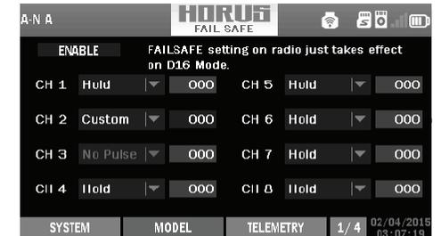
3. Failsafe can be set on receiver via short press Bind button while moving channel position to a preset value after binding.
